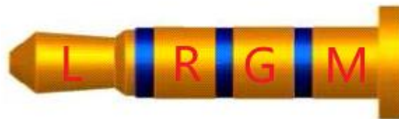
Figure 18 Definition of four-segment headphones
